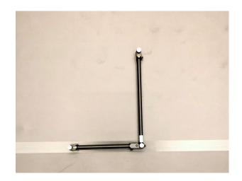
Place the L shaped ground plane in the **middle of the room**, facing the long side to the large door.
