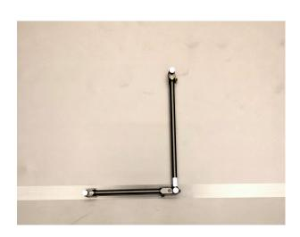
Place the L shaped ground plane in the **middle of the room**, facing the long side to the large door.
