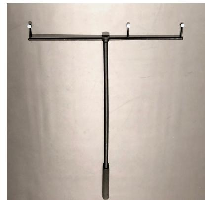
Take the passive wand (with grey reflectors), **walk trough the tracking space** and **swing the wand continuously in front of all cameras** and also in the middle of the space.
