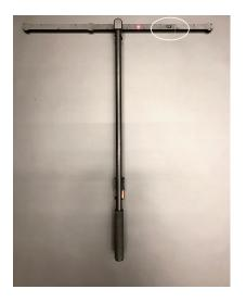
Take the active wand (with battery) and **turn it on** on the back, **walk trough the tracking space** and **swing the wand continuously in front of all cameras** and also in the middle of the space. The 3 active marker LED are on the opposite side of the On/Off switch, so make sure that they point
